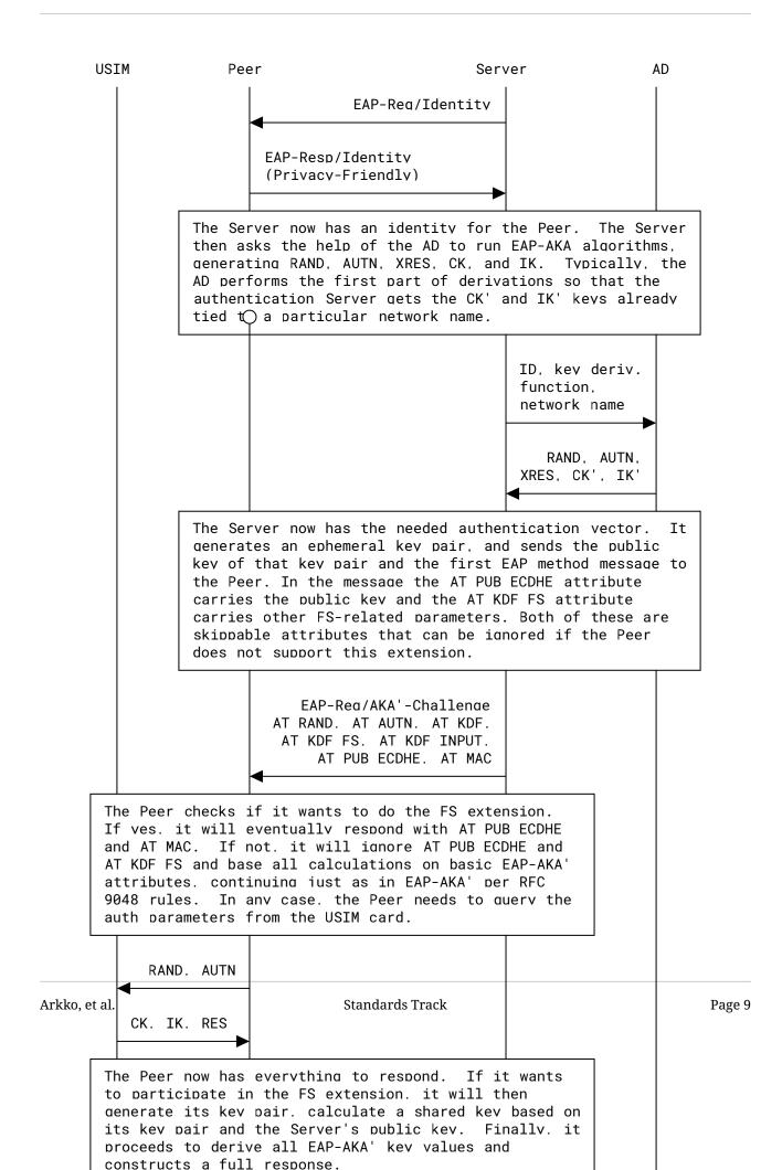
Figure 2: EAP-AKA' FS Authentication Process
