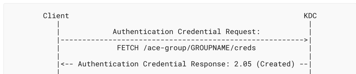
Figure 16: Message Flow of Authentication Credential Request-Response to Obtain the Authentication Credentials of Specific Group Members
